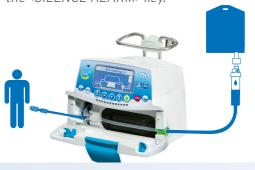
1. Align the tubing set horizontally along the tube guides so that the green connector is positioned to the right (green) and the blue clamp is positioned in front of the clamp guide (blue).
