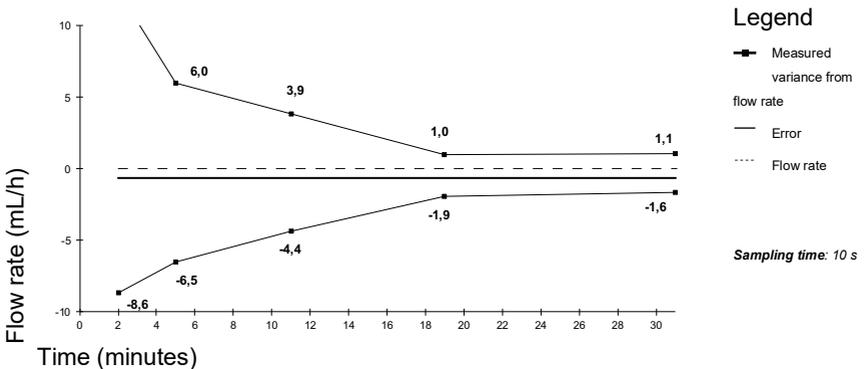
**Figure 19.7:** Trumpet curves for 2, 5, 11, 19, 31 minutes observation windows (1 mL/h over 2 hours)
