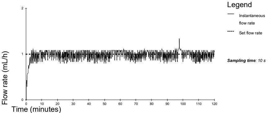
**Figure 19.6:** Start-up and instantaneous flow rate (1 mL/h over 2 hours)
