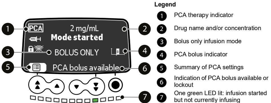
**Figure 7.1:** PCA infusion in bolus only mode (started but not currently infusing)
