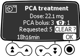
2. If you want to reset the count to zero on these indicators, press the confirm key
