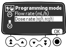
1. Use the arrow keys to select the programming mode, and press **OK** to confirm.
