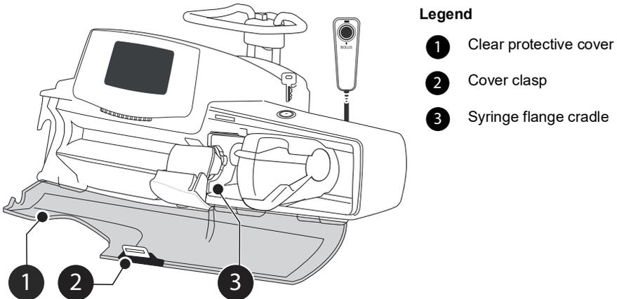
Figure 3.2: Front view with cover open
