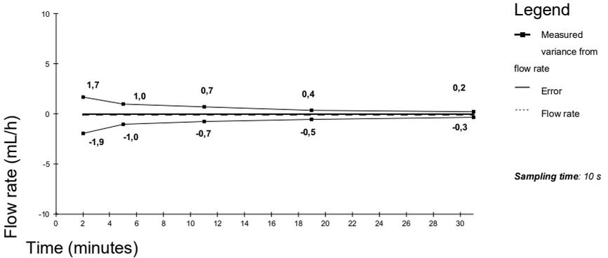
**Figure 19.9:** Trumpet curves for 2, 5, 11, 19, 31 minutes observation windows (5 mL/h over 2 hours)
