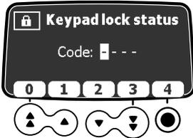
3. If a code is required, press the keys to enter the unlock code.
