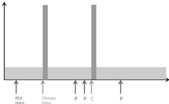
**Figure 4.2:** Continuous rate infusion mode
