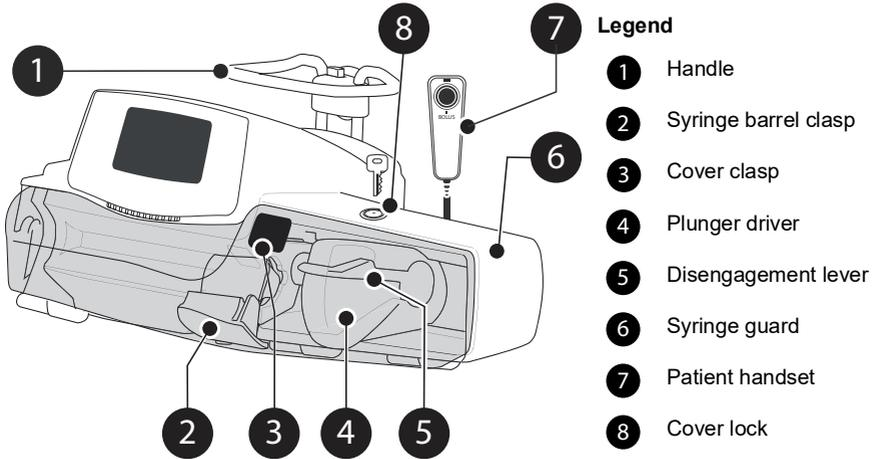
Figure 3.1: Front view with cover closed
