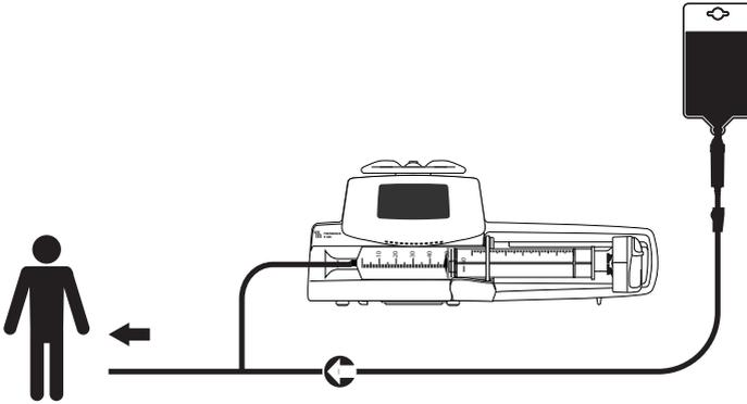
**Figure 15.1:** Gravity Infusion (in parallel with a pump)
