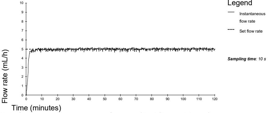
**Figure 19.8:** Start-up and instantaneous flow rate (5 mL/h over 2 hours)
