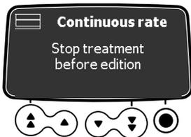
**Figure 7.4:** Alert message requiring to stop infusion
