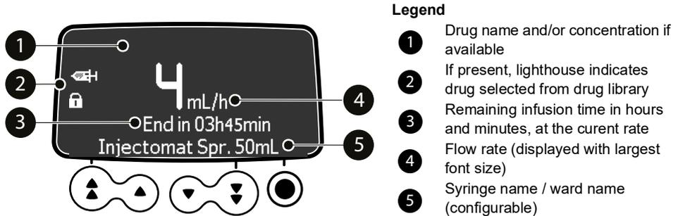
**Figure 8.1:** Infusion programmed by flow rate in progress
