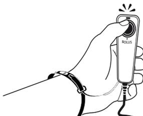
If a PCA bolus is not available due to the lockout period between two consecutive boluses, or because the maximum number of boluses allowed has been reached, on pressing the bolus button, the pump beeps and the LED on the patient handset flashes but the pump does not deliver the bolus.
