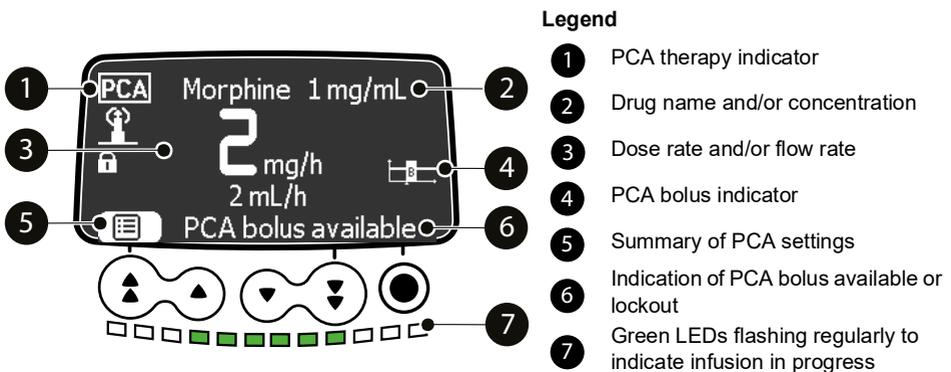
**Figure 7.2:** PCA infusion in progress in bolus + continuous mode - bolus available
