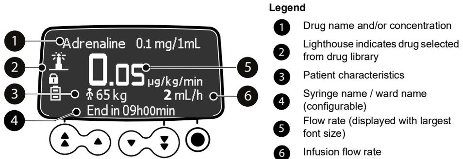
**Figure 8.2:** Infusion programmed by dose in progress
