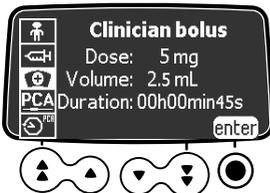
2. To modify the settings, unlock the keypad, as explained in Section 10.4, page 93. *The keypad will lock automatically again within 15 seconds.*
